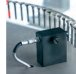
PLA 33-11, absolute probe, e.g. for material verification testing
