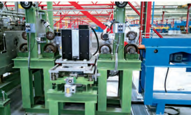
Inspecting wires / bars using encircling coils
