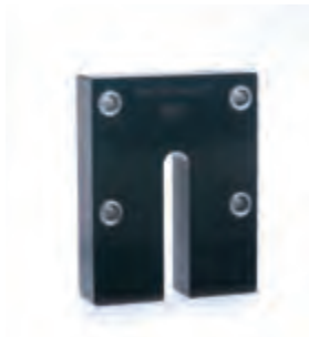
PKA-5 H-1668, transmission probe, for material verification testing
