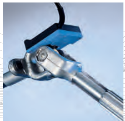
Crack detection on safety relevant structures
