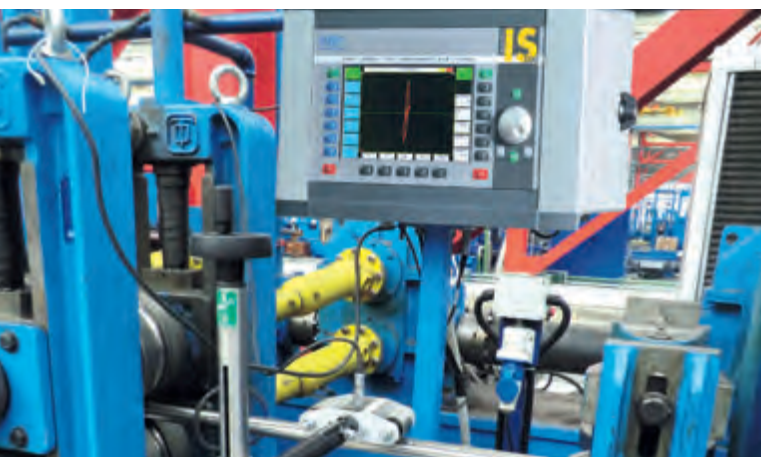
Testing the weld seam
