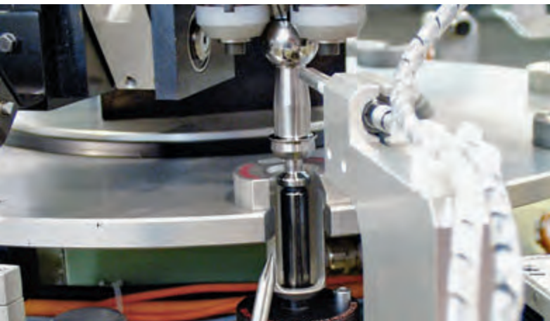
Fully-automatic crack detection on ball studs
